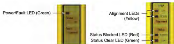
Figure 2. EZ-SCREEN Type 2 emitter and receiver status indicators
