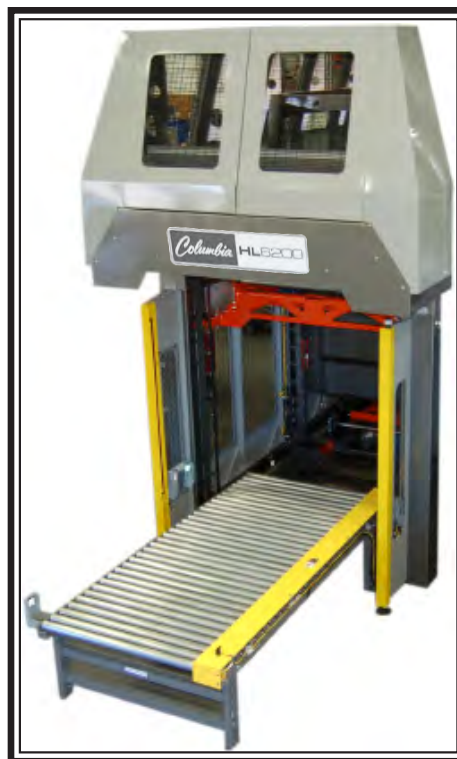
View of Lower Palletizing Section
