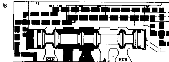
2 POSITION SINGLE PRESSURE SHOWN WITH "B" OPERATOR ENERGIZED
